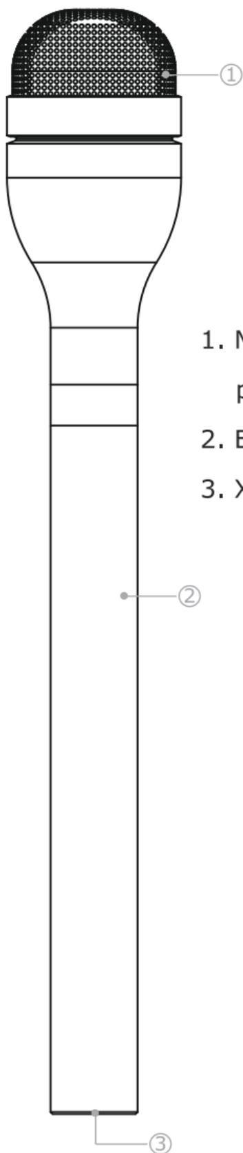
1. Mesh head with internal plosive screen
