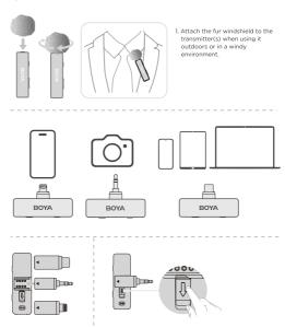
Push the selected adapter into the receiver. Connect the receiver to your audio devices, such as a camera, smartphone, tablet, computer, etc.
